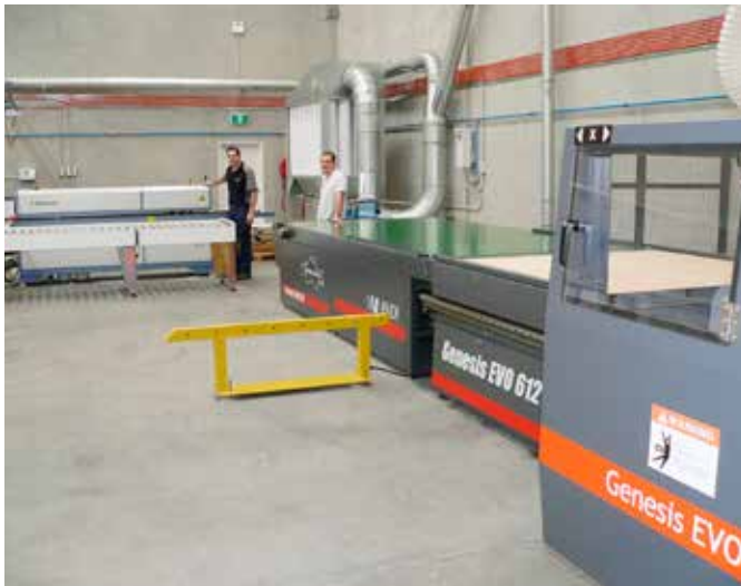
Andersen Genesis EVO 612 CNC router coupled with a Hebrock F4 edgebander set up to produce twenty kitchens a week.
