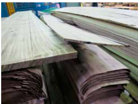
The remnants: on the left after slicing with mechanical clamps, on the right with vacuum clamps.
