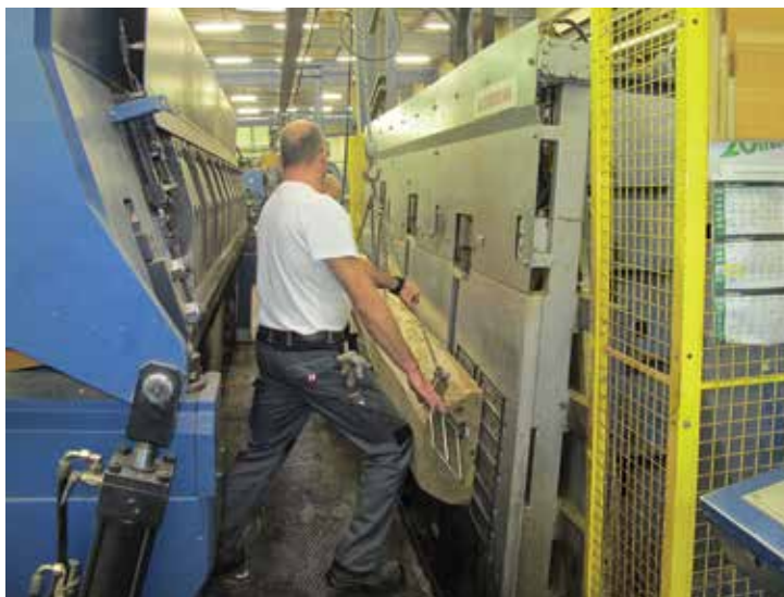
Adjusting of a flitch on the clamping device
