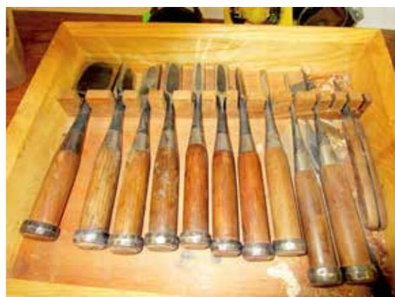
will reflect in the accuracy, finesse, and quality of the finished work. Another feature is the use of laminated steel, one layer of soft and one layer of hard steel. "If you use only hard steel, the tool becomes quite brittle, and also it takes a lot of time to sharpen. The hard steel, when you hit it, can crack or nick very easily but soft steel acts like a shock absorber, and generally speaking the hardness of Japanese steel is very strong."
