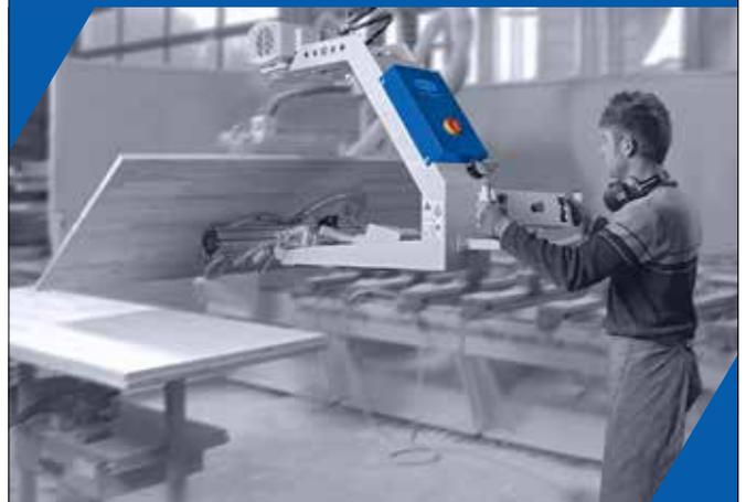
**THE VACUMASTER 180° VACUUM LIFTER** ALLOWS A HORIZONTAL LOAD TO BE LIFTED AND ROTATED 180° BY **A SINGLE OPERATOR**
