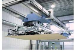
more manual handling necessary. The TLF sets the program a night before, picks orders over night and is ready for production the next morning. This all-rounder for a wide variety of panels is available as stand-alone or integrated cell solution.
