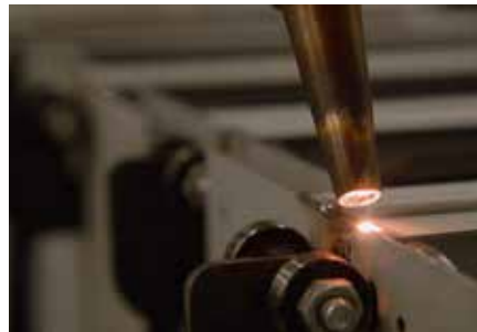
Laser welding of Concelo components.
